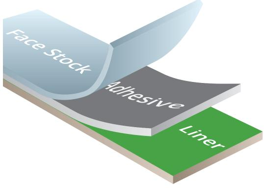
**Adhesive:** 0.7 mil ultra removable acrylic adhesive designed for high initial tack with clean removability when needed.
